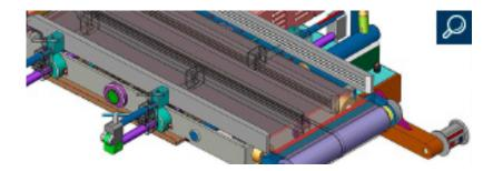
The Quick Change Over feature is a lateral guide immediately in front of the blade. It is powered by a motor and automatically adjusts to different widths of product - a particular advantage with products of different widths. This automatically improves the slicing quality achieved, particularly if you change or vary your products frequently.
